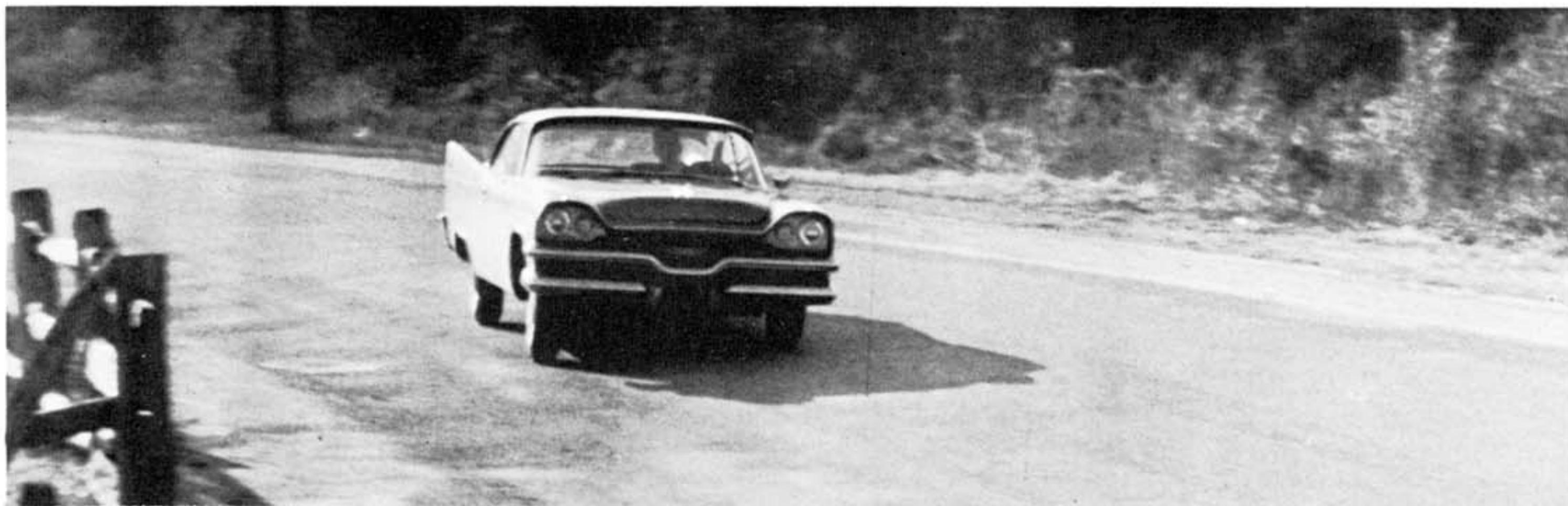
In SCI's fastest test bend, D500's speed and controllability compared favorably with general run of production sports cars. Leaning only moderately at 75 mph, front wheel outward camber is not excessive.
